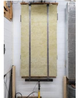
Fig. 2 Test Specimen Wall Installed
